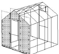
NOTE: When trimming off portions of Solexx paneling during the end wall paneling installation, you should leave an extra 1/8" (3mm) of the paneling above the framing that you are using as a cutting guide. This allows the end wall paneling to "snug" up against the side walls and roof paneling. Once the paneling is attached and trimmed, seal all open ends of the paneling with 100% Silicone caulking.
